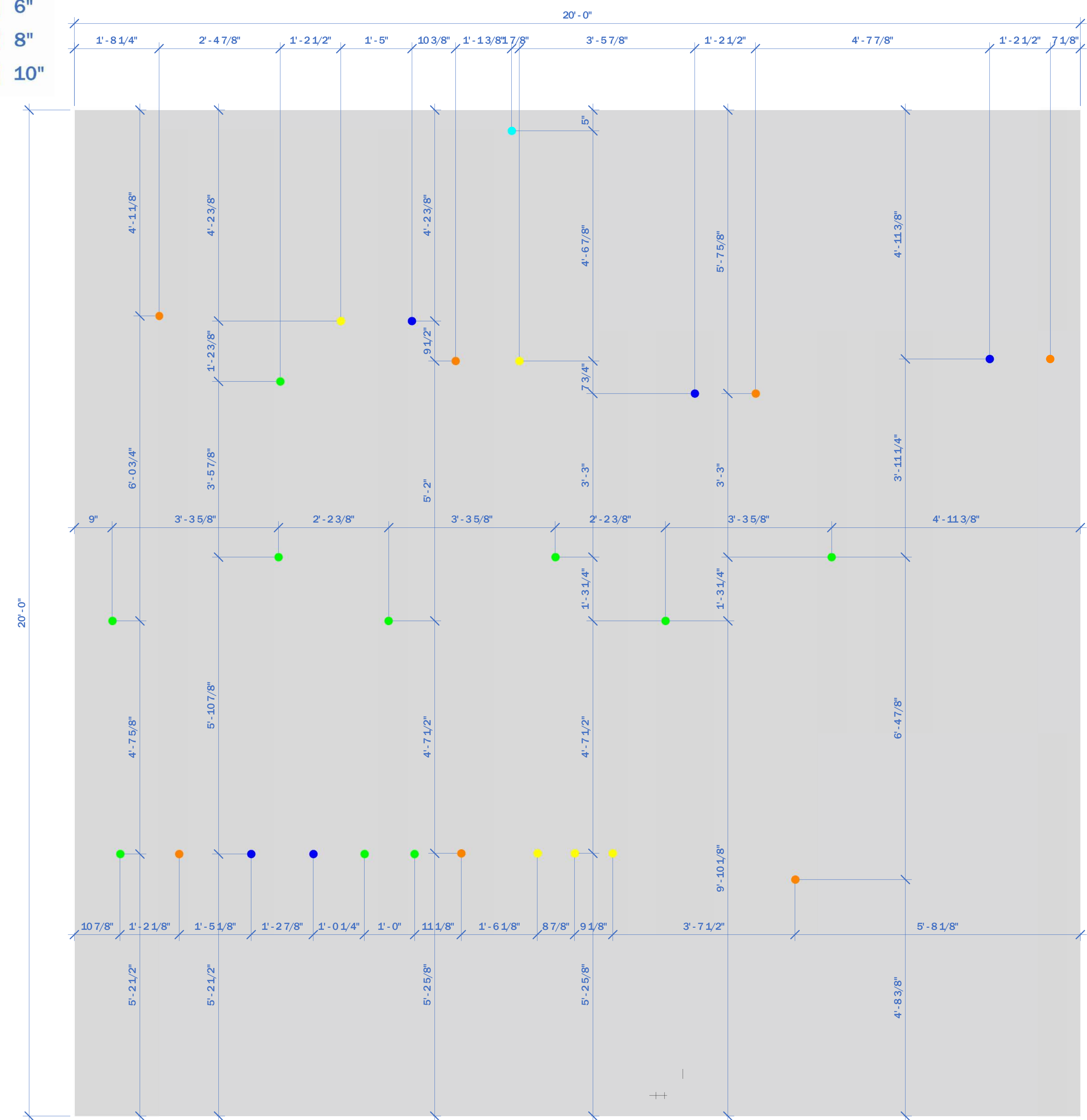
① EQUIPMENT STUB-UP PIPING PLAN 3/4" = 1'-0"
